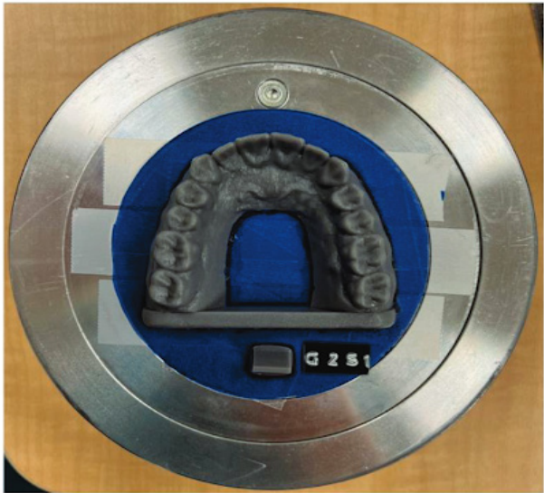
3D-printed model and geometric form pair oriented on the flat platform of the Biostar thermoforming machine utilizing a placement guide.
